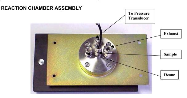
Figure 6A Reaction Chamber Assembly (Oven Side)
