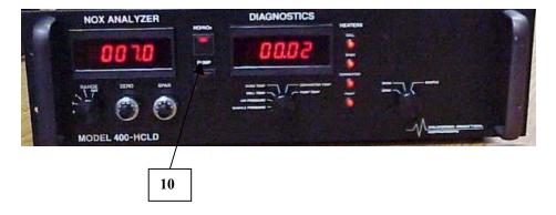
Figure 2B: Front Panel (Pump Version)
