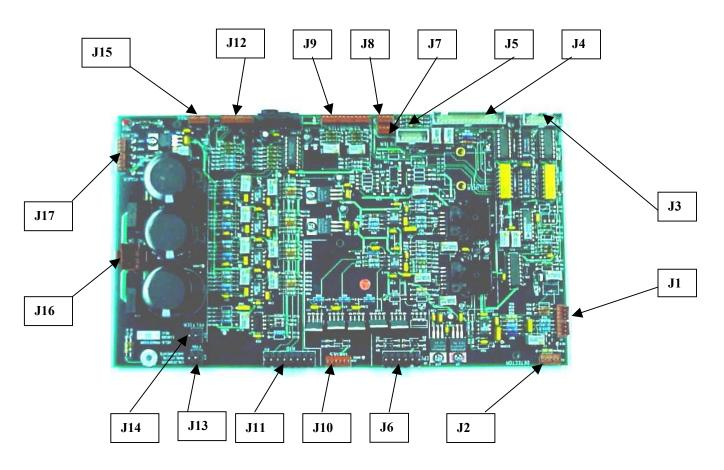
**Figure 5B** Main Electronic Board Components (Connectors)
