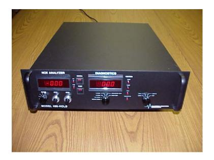
This manual describes installation, calibration and operation of California Analytical Model 400 HCLD heated oxides of nitrogen gas analyzer. To assure correct operation and accurate results, it is recommended that the user carefully read this document.
