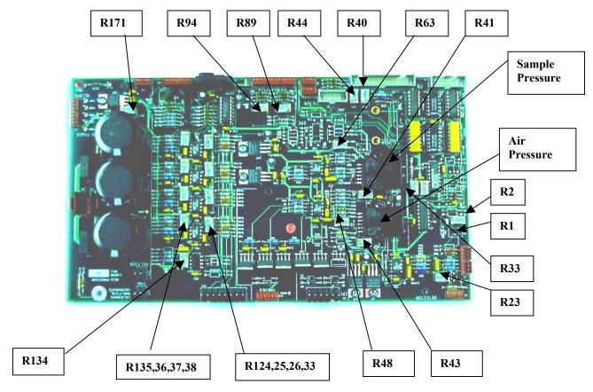
Figure 5A Main Electronic Board Components (Potentiometers)
