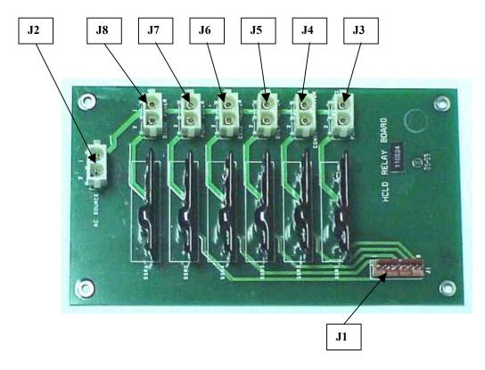
Figure 7 Relay Board Connections
